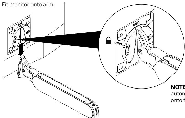
**NOTE:** VESA head will automatically latch onto the tilt link
