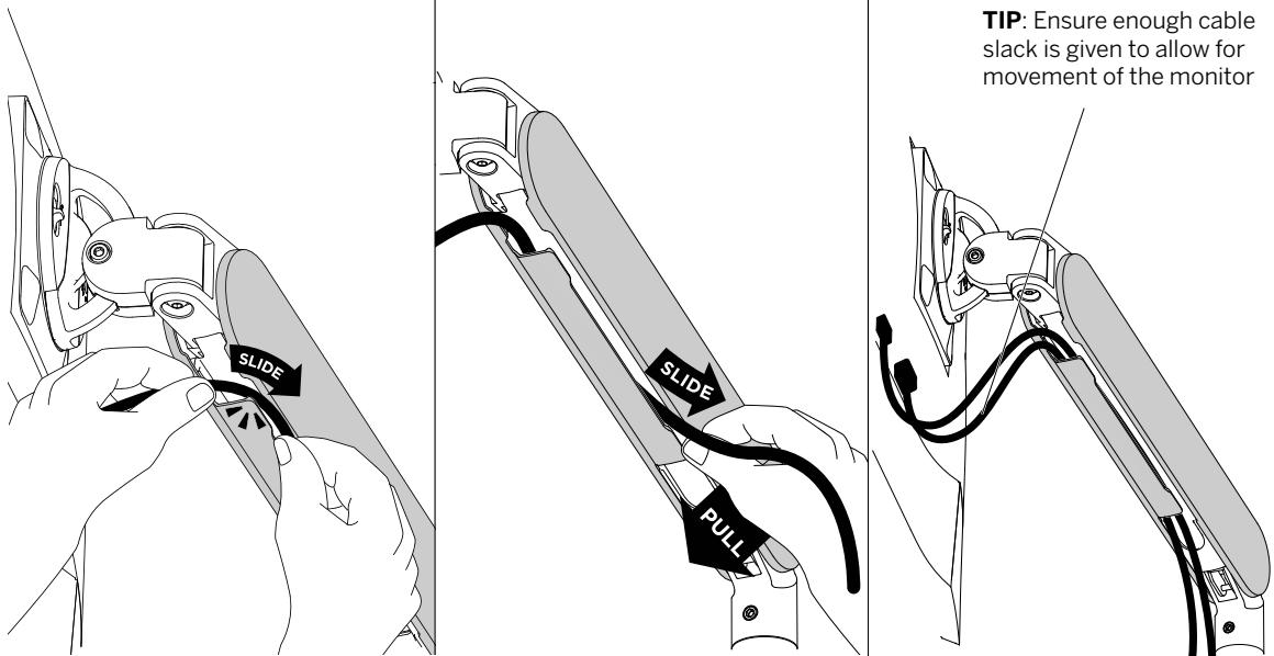
Plug cables into lower arm hook flaps
