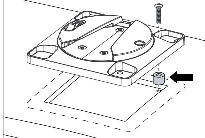
Attach VESA head onto monitor with provided screws.
