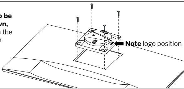
**Note:** Ensure screw length suits the monitor VESA mounting holes
